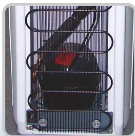
Hermetically sealed reciprocating compressor
